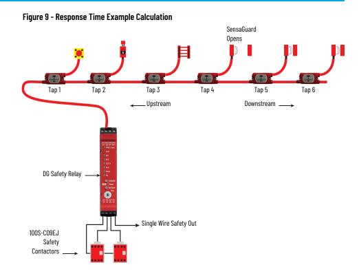
The safety system response time for the system that is shown in <u>Figure 9</u> is listed in <u>Table 7</u>. The time from when the SensaGuard interlock opens to the time when the 100S contactors drop out is 169.105 ms. The time from when the SensaGuard interlock opens to the time when the SWS signal turns OFF is 114.105 ms.
