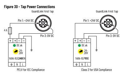
Figure 30 shows the power connections to the power tap. Power is connected only to the first tap.
