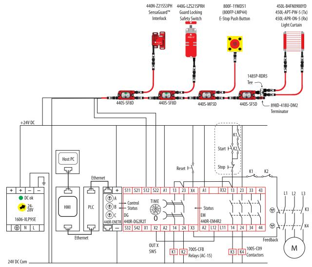
This system has eight safety functions; two functions for each input device. One function is for the DG outputs, and the second is for the expansion module outputs. The safety Function Block Diagrams are shown in Figure 46.
