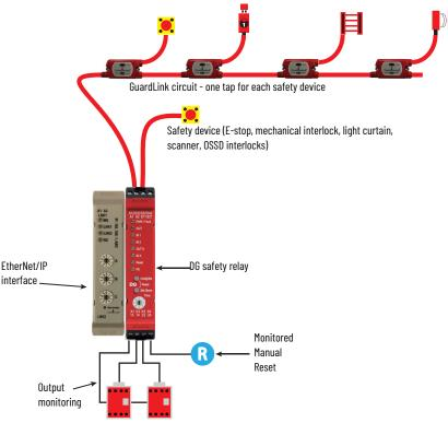
Figure 3 shows an example of a DG safety relay operating as the equivalent of a DI safety relay. In Figure 3, the DG safety relay is configured to accept two input devices, control and monitor two contactors with a manual reset input. The 440R-ENETR interface reports the status to the machine control system. The machine control system can also initiate a reset command.
