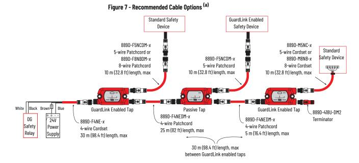
(a) Replace the *x* with 0M3 (0.3 m [0.984 ft]), 0M6 (0.6 m [1.968 ft]), 1 (1 m [3.28 ft]), 2 (2 m [6.56 ft]), 5 (5 m [16.4 ft]), 10 (10 m [32.8 ft]), 15 (15 m [9.2 ft]), 20 (20 m [65.6 ft]), or 30 (30 m [98.4 ft]) for standard cable lengths.
